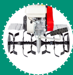
ROTAVATOR riveted knives Ø32 cm 75 cm can be reduced to 50 cm with discs
